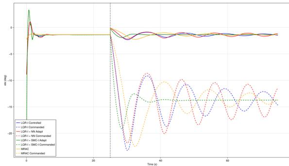
Fig. 19. Elevator Adaptive Controller Responses with 90% Loss of Elevator Effectiveness. The dashed lines represent the commanded deflection.
