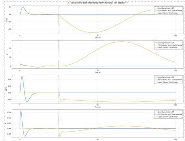
Fig. 4. PID Performance With loss of elevator effectiveness
