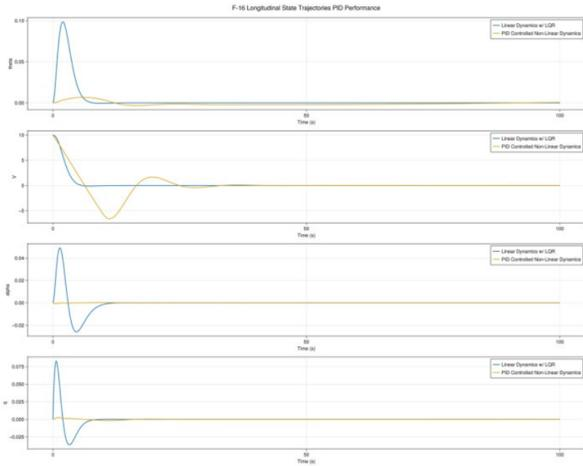
Fig. 3. PID Performance Without Disturbance
