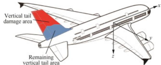
Fig. 2. Airplane vertical tail failure [7]
