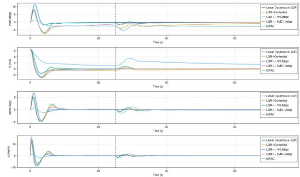
Fig. 16. Adaptive Controller Comparison with 50% Loss of Elevator Effectiveness and LQR-I Base Controller.
