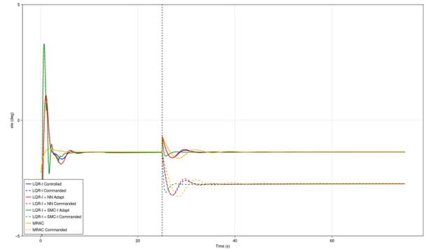
Fig. 17. Elevator Adaptive Controller Responses with 50% Loss of Elevator Effectiveness. The dashed lines represent the commanded deflection.
