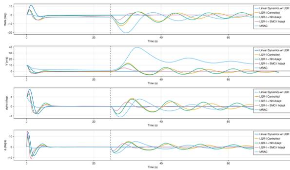
Fig. 18. Adaptive Controller Comparison with 90% Loss of Elevator Effectiveness and LQR-I Base Controller.
