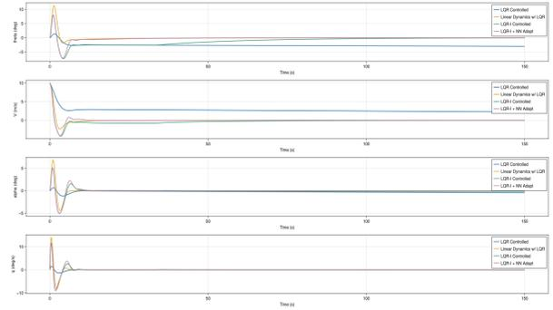
Fig. 12. NN Adaptive Control Response Without Disturbance
