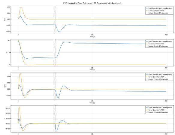
Fig. 6. LQR Performance With loss of elevator effectiveness
